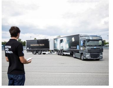
The ZF Innovation Truck – a truck prototype with a length of over 25 meters – can be conveniently maneuvered via tablet remote control with zero local emissions. Source: ZF FRIEDRICHSHAFEN AG
