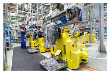
8-speed automatic transmissions for passenger cars are produced at ZF's location in Saarbrücken. Source: ZF FRIEDRICHSHAFEN AG
